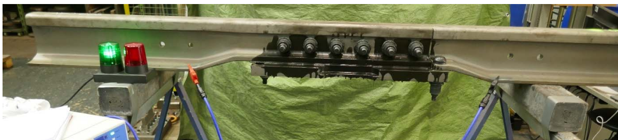
Figure 9: Measurement of electrical insulation between connected rail profiles
