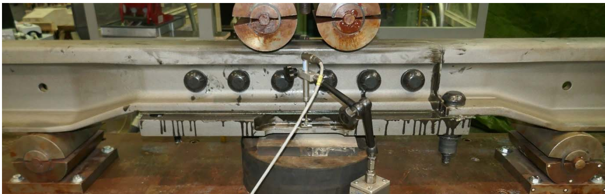
Figure 6: Sample ABJ-008 in the test set-up of the bending fatigue test
