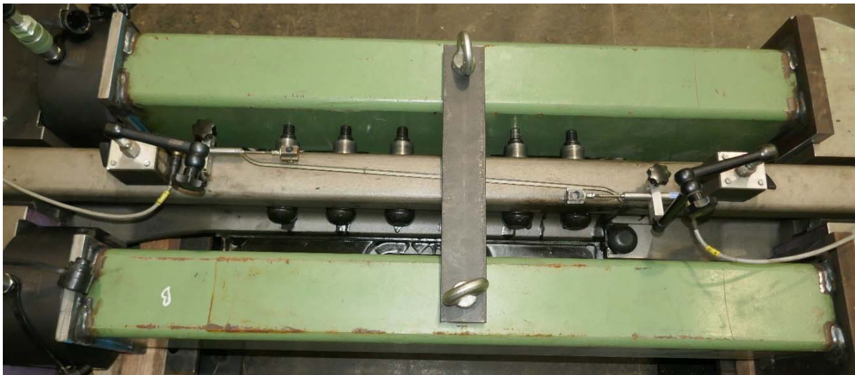
Figure 5: Sample ABJ-007 in the test set-up to verify the longitudinal load transmission
