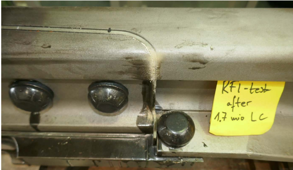
Figure 7: View of the butt joint after 1.7 million load cycles
